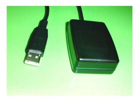
The GM-R307 GPS receiver provides EverMore's latest 12-channel GPS technology, contained inside a mouse-like box with a host connection cable.
