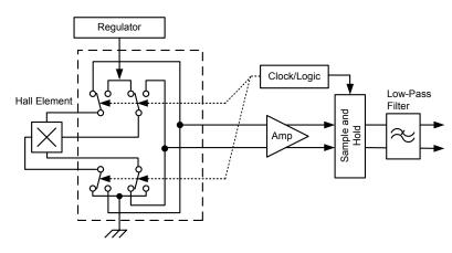
Concept of Chopper Stabilization Technique
