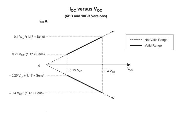
Example: For ACS710KLATR-6BB-T, if required overcurrent fault switchpoint is 10 A, and  $V_{CC}$  = 5 V, then the required  $V_{OC}$  can be calculated as follows:
