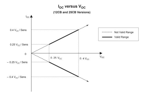
Example: For ACS710KLATR-25CB-T, if required overcurrent fault switchpoint is 50 A, and  $V_{CC}$  = 5 V, then the required  $V_{OC}$  can be calculated as follows:
