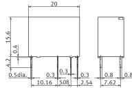
General tolerance Less than 1 mm:  $\pm 0.2$ Min. 1 mm less than 5 mm:  $\pm 0.3$ Min. 5 mm: ±0.4
