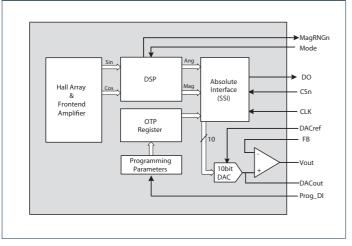
The analog output can be configured in many ways, including user programmable angular range, adjustable output voltage range, voltage or current output, etc. An internal voltage regulator allows operation of the AS5043 from 3.3V or 5.0V supplies.
