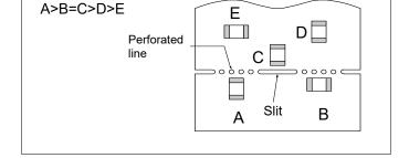
to varistor placement, consider the board breaking method as well.
