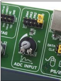
Figure 11-1: ADC (default jumper positions)
