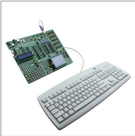
Figure 9-4: EasyAVR6 connected to keyboard
