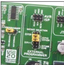
Figure 4-1: Setting jumper J7
