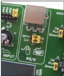
Figure 9-1: PS/2 connector (J16 and J17 are not placed)
