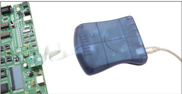
Figure 5-2: JTAGICE mkII connected to the development system
