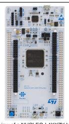
Top view of a NUCLEO-L4XXZY board without Ethernet peripheral.
