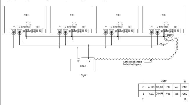
Note : In parallel connection, maybe only one unit (master) operate if the total output load is less than 5% of rated load condition. The other PSUs (slaves) may go into standby mode and their output LEDs will not turn on.
