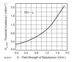
Figure 8. Sensitivity vs. Electric Field Disturbances
