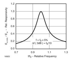
Figure 5. Frequency Dependence of Responsivity
