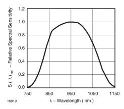
Figure 11. Relative Spectral Sensitivity vs. Wavelength
