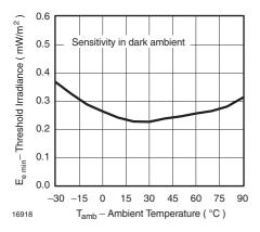
Figure 10. Sensitivity vs. Ambient Temperature
