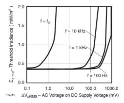
Figure 7. Sensitivity vs. Supply Voltage Disturbances
