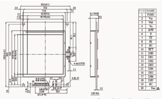
The non-specified tolerance of dimension is ±0.3mm.
