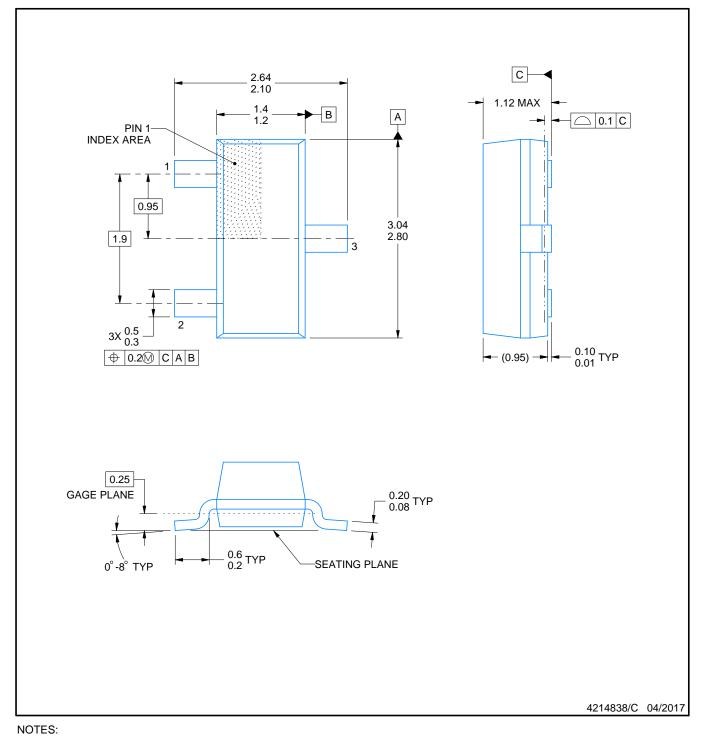
All linear dimensions are in millimeters. Any dimensions in parenthesis are for reference only. Dimensioning and tolerancing per ASME Y14.5M.
