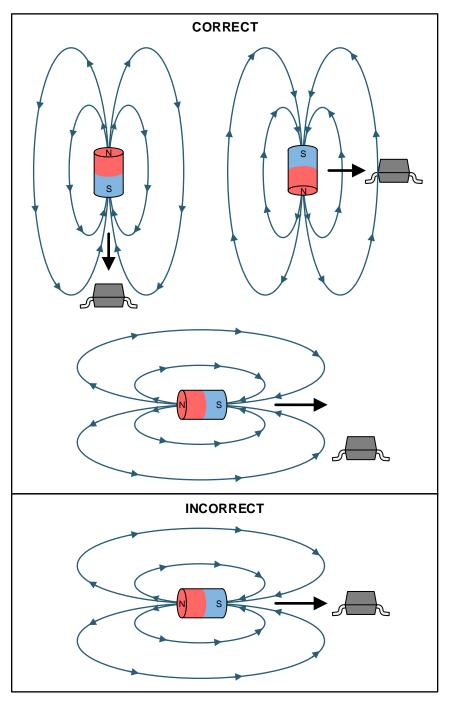
Figure 16. Correct and Incorrect Magnet Approaches
