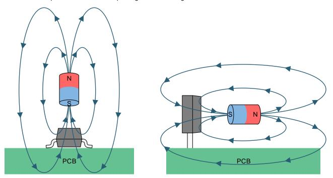
Figure 9. The Flux Direction for Positive B
