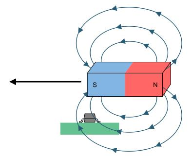
Figure 14. Common Magnet Orientation
