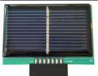
**MSP430-SOLAR** is power supply module with solar panel and rechargable battery. The solar panel is rated 2.4V 80mA and have on board DC/DC voltage boost converter which generates 3.3V for the MSP430 target. The board have female 2x7 IDC keyed connector which can be
